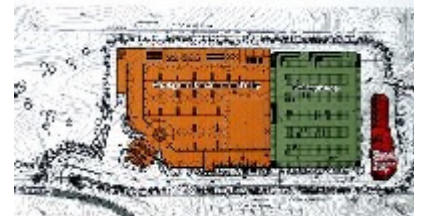
An overview of the proposed Buena Vista casino shows the gaming and entertainment facility, orange; parking garage, green; and water and wastewater treatment facility, red. Coal Mine Road is depicted in the lower left-hand corner.
